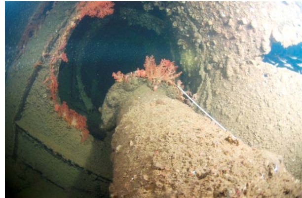
Flange B, now just inside hull where stern tube should be, is the only remaining intact flange on entire shaft.
