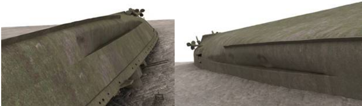
Left. Starboard side hull indentation (also see Figures 7 and 10). Right. Port side hull indentation (also see Figures 7 and 9).
