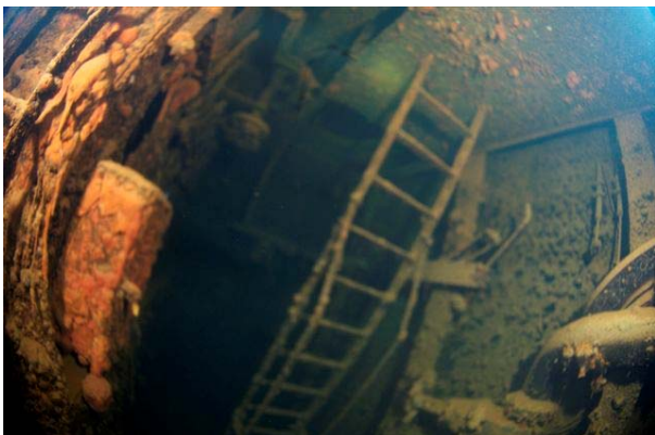
Alcove on outboard side of the Thrust Block enclosure. Behind ladder is the bulkhead to B Engine Room, Frame 184. Under the 'drum' in image on right is a deckhead hatchway.
