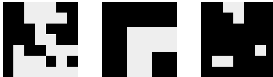
Figure 7.8: Binary erosion. (left) data, (middle) structure element, origin in centre, (right) eroded output.
