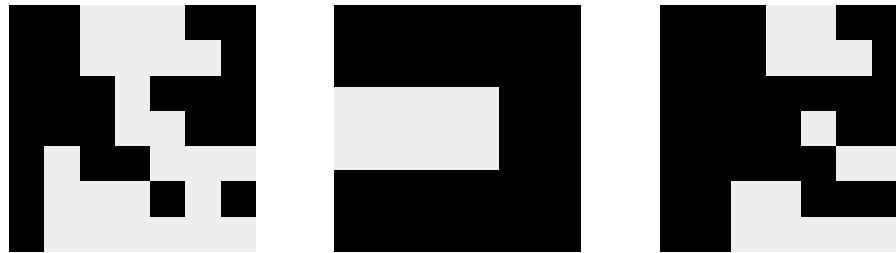
Figure 7.7: Binary erosion. (left) data, (middle) structure element, origin in centre, (right) eroded output.
