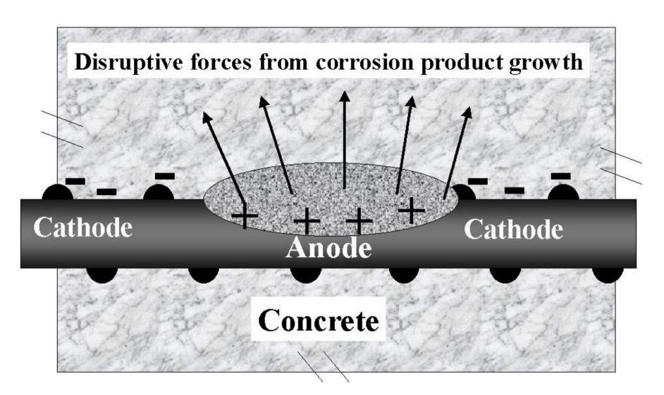
Figure 1. Schematic of embedded reinforcement corrosion cell
