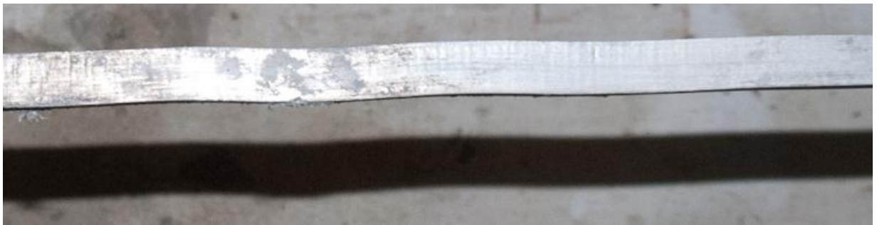
Figure 29 – Visible residual plastic deformation showing that local buckling occurred around the weak axis
