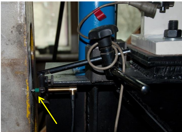
Figure 9 – Device used for measuring horizontal displacement
