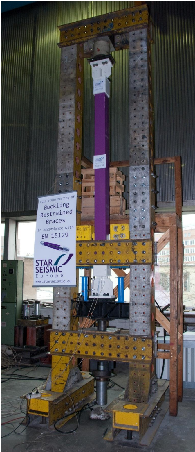
Figure 7 – BRB test setup
