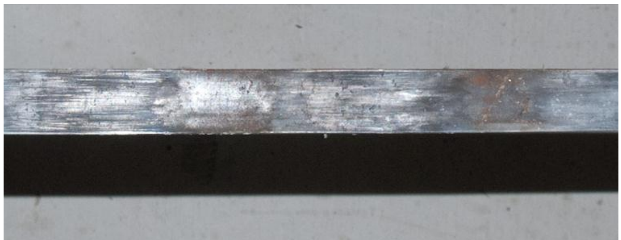
Figure 30 – No sign of residual deformation from local buckling around the strong axis
