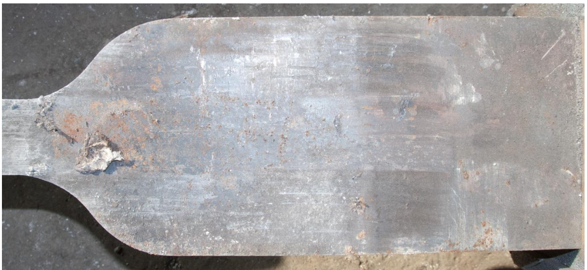
Figure 33 – Elastic and transition zones of the steel core show no damage
