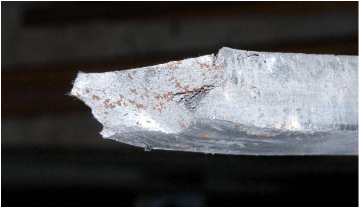
Figure 32 – Rupture surface of the steel core
