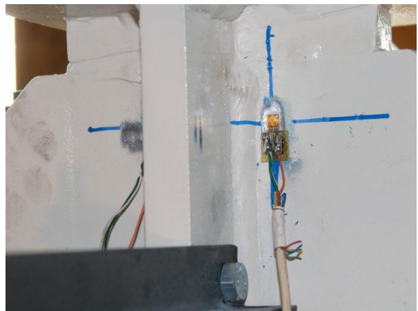
Figure 10 – Gauges installed on the subassembly structure
