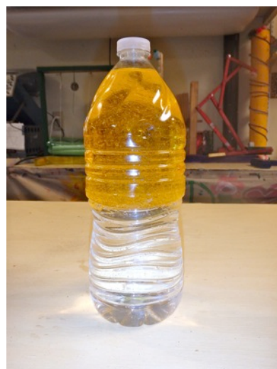
Carefully pour oil on top of the water until the bottle is nearly full.
