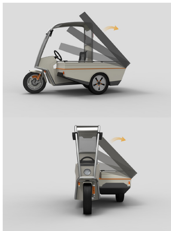
Figure 9.7 Tilting of the platform
