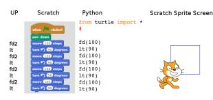
Figure 3. Matching Program structures in UP, Scratch and Python: drawing a square
