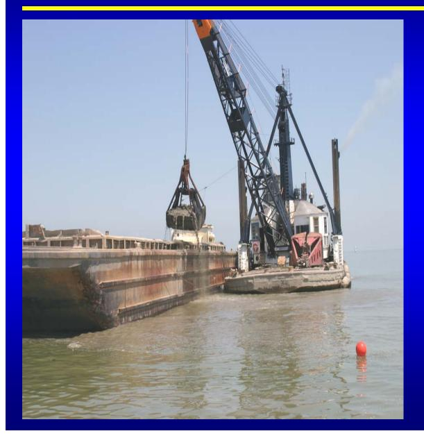
**Characterize the** spatial extent, concentration gradient structure, and temporal dynamics of suspended sediment plumes during bucket dredging operations.
