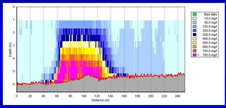
Near-field plume conditions immediately after sediment release. Peak TSS concentrations 1,100 mg/l
