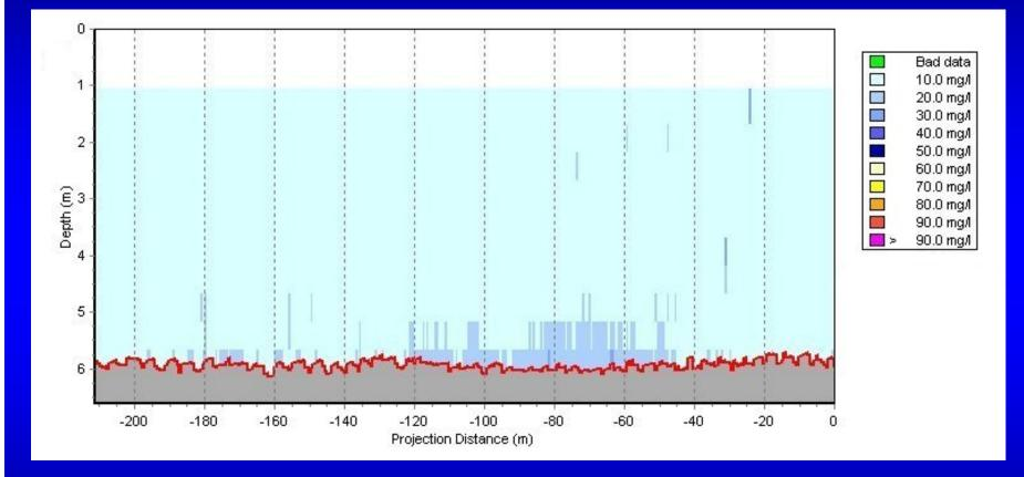
• Traces of plume signature remain on bottom at 265 m northeast of the release point
