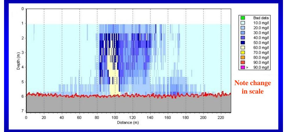
Maximum TSS concentration 70 mg/l at 215 m northeast of the release point
