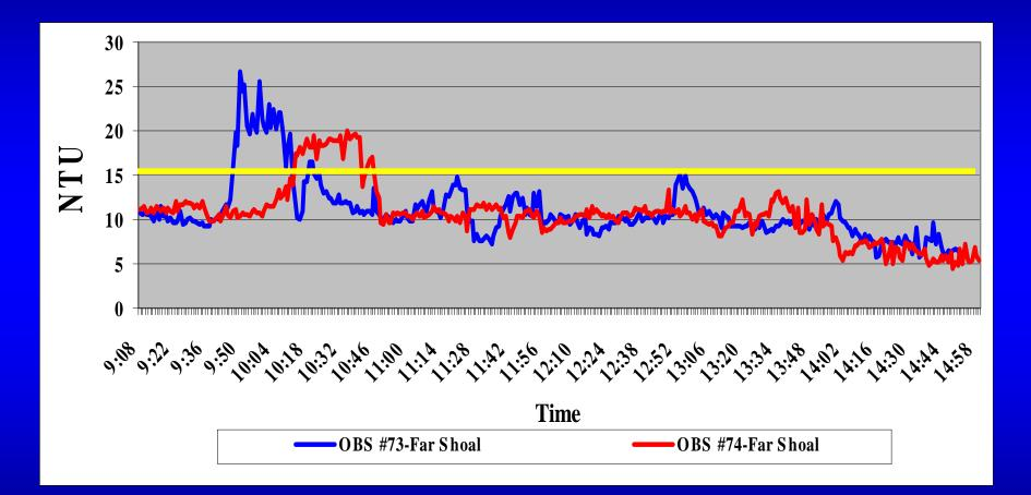
• Sensors deployed further from the channel and dredge during a 6 hour monitoring segment (OBS units at # 74 at 120 m and #73 at 160 m).
