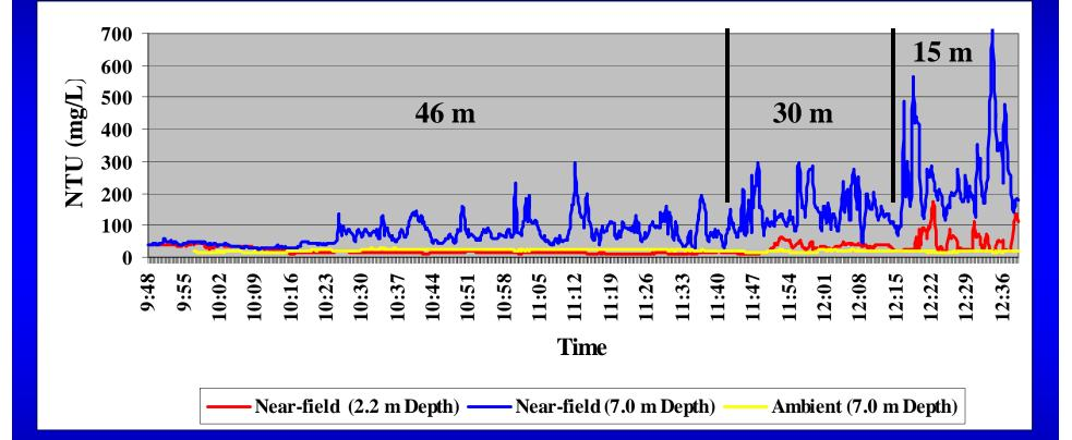
Peak Lower Water Column Turbidity: 700 NTU (15 m) < 300 NTU (30m) Peak Upper Water Colum Turbidity: 175 NTU (15 m) 50 NTU (30m) Ambient in < 50 m
