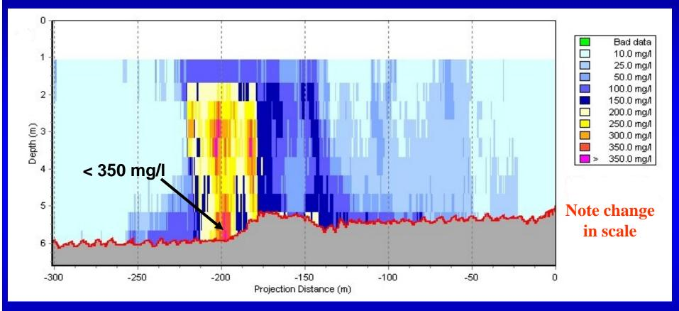
The bulk of the material released plunged directly to the bottom as a dense mass. TSS concentrations decreased by a factor of 2 in comparison with previous transect.
