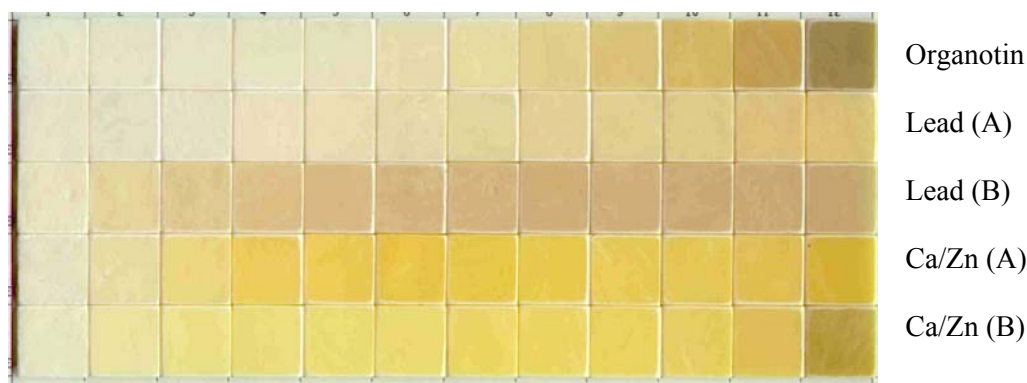
Figure 5.1: Heat stability - 2-roll mill @ 200°C - 1 min. intervals
