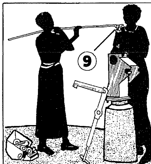
Figure 4.1: The Afridev Handpump scheduled maintenance card: front
