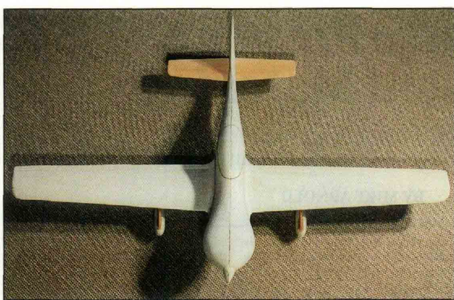
AR-6 Formula 1 design, showing engine cowl fairing in to fuselage sides over point of max. thickness on wing. Fuselage sides are then parallel back to trailing edge.
