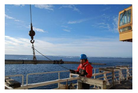
ii. Lower the barrel to the water until the lower end breaks the surface. Using a deck hose, fill the core barrel with salt water until COMPLETELY full.<sup>1</sup>
