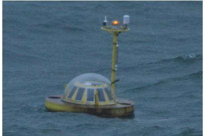
Figure 1-42. Wave Rider Buoy
