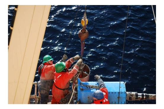
vi. With the 04 crane, maneuver the core up and clear of the Aframe. Assist in guiding the core upward and attach the lower tagline, and cap the end once the core exits the water (this ensures no loss of sediment).<sup>1</sup> Disembark the Hero Platform and replace lifelines.<sup>1</sup>
