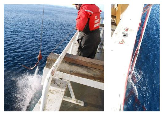
iv. Notify the bridge that the core barrel is in the water.
