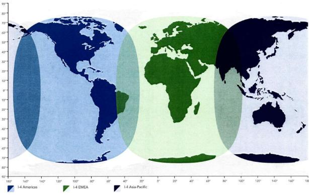
Figure 2-1. INMARSAT B FBB Satellite Coverage
