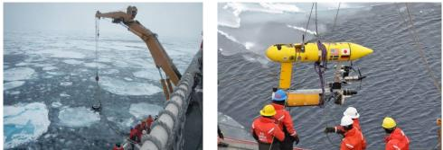
Figure 1-28. HEALY Deck Division deploys the VOBSS (left) and UUV (right)
