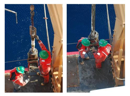
vi. Using the HIAB crane (wire rope), take the weight of the trigger arm and, using an impact wrench, disconnect the bolts holding the trigger arm to the 9/16" wire.<sup>1</sup>
