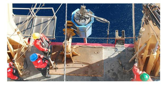
(2) The HIAB Crane, Core Barrel Rack and Pig Weights are placed around the starboard working deck as shown.
