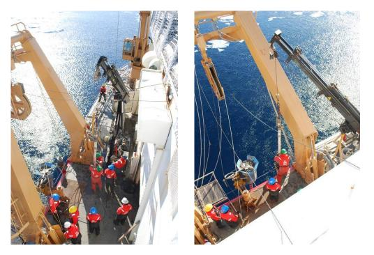
vi. Once the trigger core is seated in the weight stand, attach the core to the weights using the collar and bolts.<sup>1</sup>
