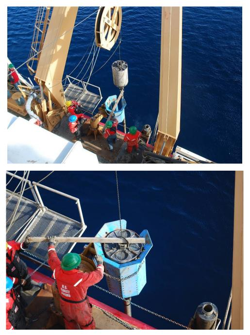
the core barrel to align properly (lifting ring parallel to the hull, lifting point on weight barrel facing aft).<sup>1</sup>
