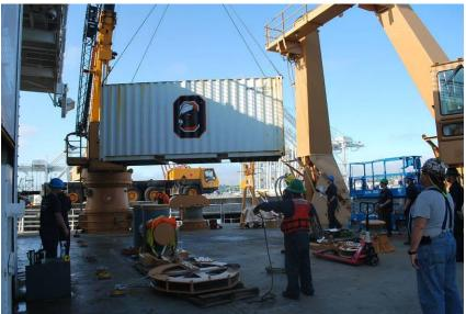
Figure 1-1. The first of three coring vans is loaded onto the fantail in Seattle via the Ness Crane
