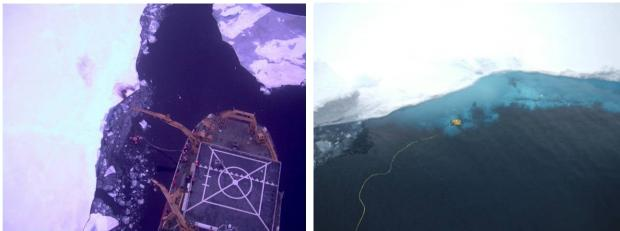
Figure 1-30. (Left – photo taken by sUAS) HEALY deploys the skimmer to clear mock oil from near an ice floe (Right) The ROV searches for mock oil near the ice edge
