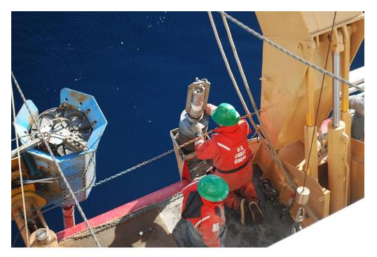
vii. Take in the 9/16" wire until it takes the load of the trigger arm. Rotate the trigger arm outboard (a 2x4 can help with this).<sup>1</sup>
