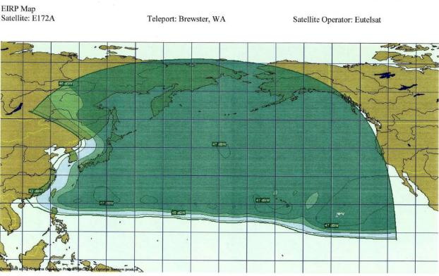
Figure 2-2. INMARSAT Ku-Band E-172A North Pacific Beam Coverage
