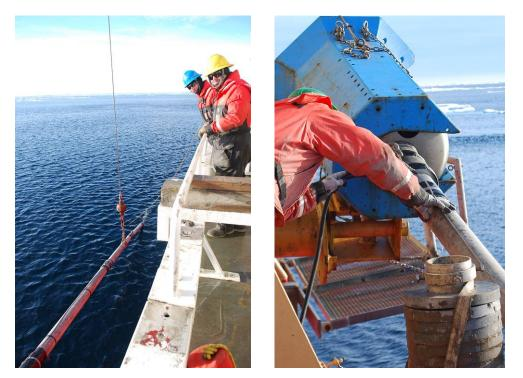
iii. Once full, consult with the Science Coring Technician and pull the quick release. The core barrel will now rotate at the pivot to the vertical position.
