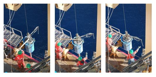
xi. A-frame out, slightly, as required for the HIAB crane to spot over the trigger core.
