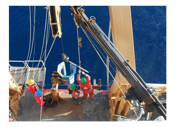
iv. Using the HIAB crane, lift the trigger core out of the water and position it in the trigger core stand.<sup>1</sup> Remove the four bolts and disconnect the weight collar from the core, and secure the weights to the stand using a ratchet strap.<sup>1</sup>
