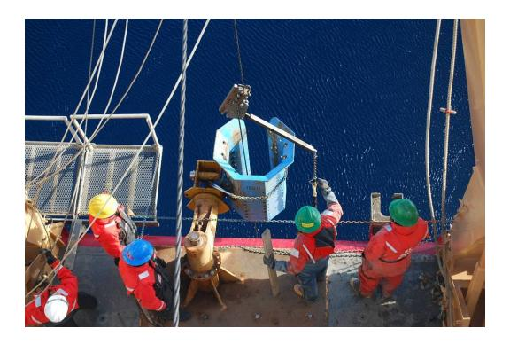
iii. Rotate the trigger arm until the trigger line sits near the trigger core stand.<sup>1</sup> Using the HIAB crane, take the weight of the trigger core and disconnect it from the trigger arm.<sup>1</sup>
