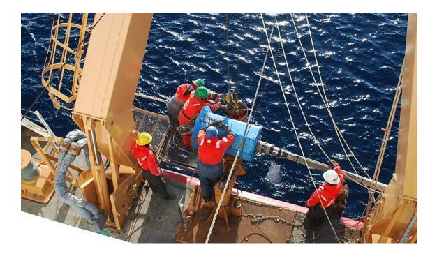
v. Transfer the load to the crane using the same sling configuration as before.<sup>1</sup> Unhook the 3/8" wire and stow.<sup>1</sup> Install the upper tagline (if required by conditions).<sup>1</sup>
