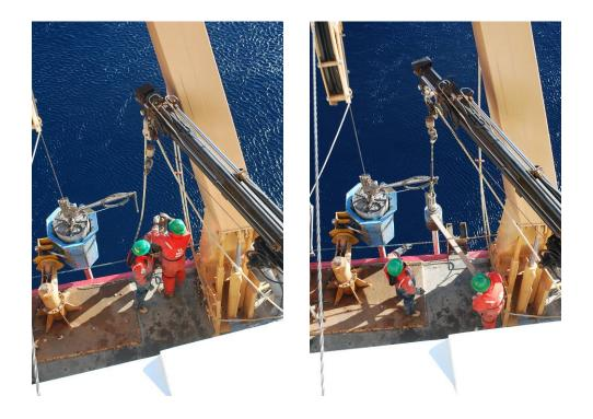
xiii. Transfer the weight of the trigger core from the HIAB crane to the trigger arm.<sup>1</sup> Separate the links in the rope and take rope back to spool on HIAB crane.<sup>1</sup> You are now ready to deploy the jumbo piston core.
