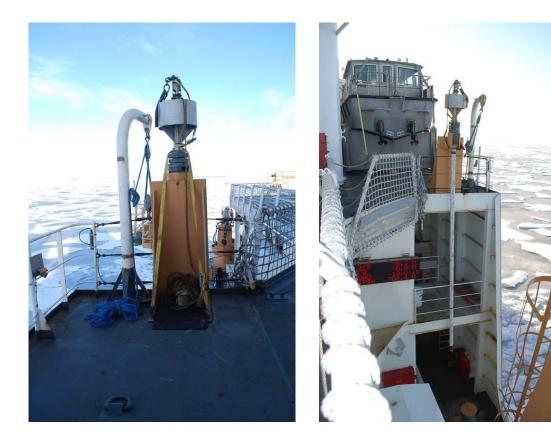
ii. Spot the starboard 04 crane (auxiliary block) over the gravity core. Sling in a basket configuration or as best determined by the Deck Supervisor. Confirm with the Science Coring Technician the exact weight of the core. However, empty, the gravity core (20 feet of pipe) typically weighs approximately 700lb, and when full of sediment, weighs approximately 1,200lb.
