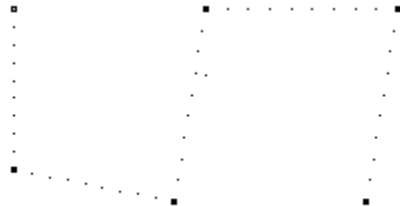
5 segments with 10 points per segment. End points are covered by the control points.
