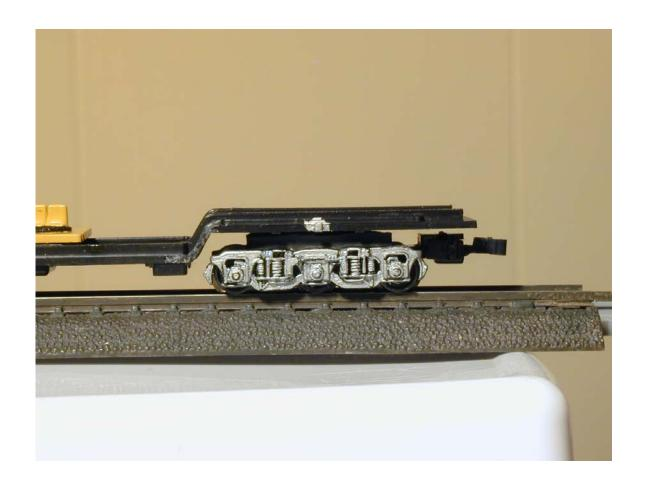
The coupler is a standard Kato knuckle coupler, filed at a slight angle to allow it to 'droop' down to the proper level to mate with other Kato Santa Fe passenger cars.
