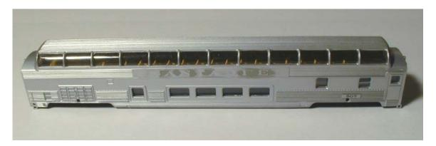
The paint underneath will come with it, but it's easily re-covered with Pollyscale Stainless Steel acrylic paint, I brush-painted it. Then re-decal using any Microscale Santa Fe streamlined passenger car decal, such as 60-4190, there are others:
