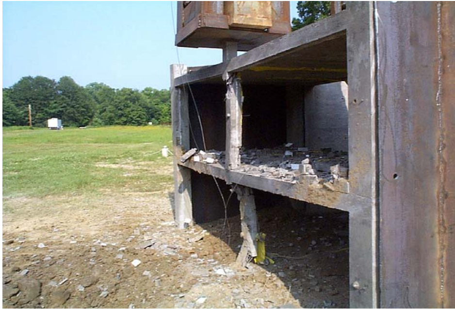
Figure 2. Post-test view of dynamic structural collapse experiment
