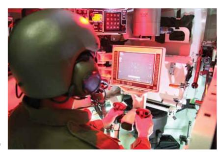
The MBT has many hardware and software configuration items each of which has their own distributed software architecture and the Vehicle Control System is the main gateway used to connect the systems to each other by means of Otokar's specially designed data interchange protocol.
