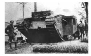
The idea was that if grenades were thrown onto the tank they would roll off again before they exploded, rather similar to the net and slat armour solutions integrated on board Mine Resistant Ambush Protected (MRAP) vehicles during the recent Iraq and Afghanistan campaigns, designed to stop rocket-propelled grenades.
