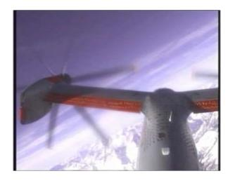
Thick wing design, resulting from dynamics requirements, produces benign stall behaviour
