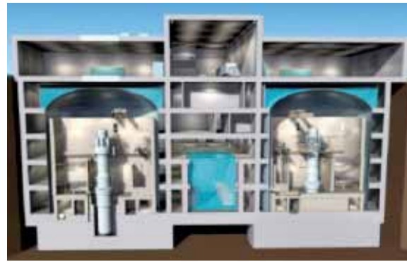
mPower containment design.
