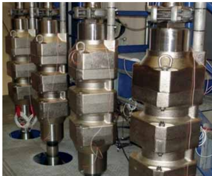
Internal control rod drive mechanism testing.
