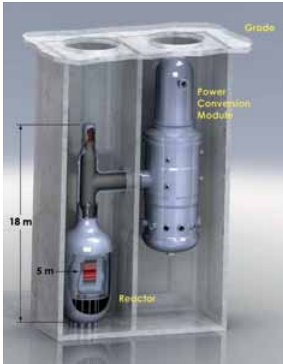
EM 2 reactor and gas turbine.
