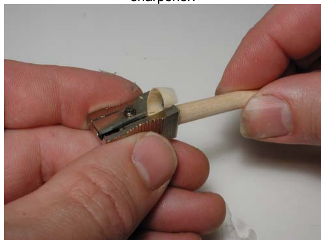
9. Sharpen the end of the dowel using the pencil sharpener.
