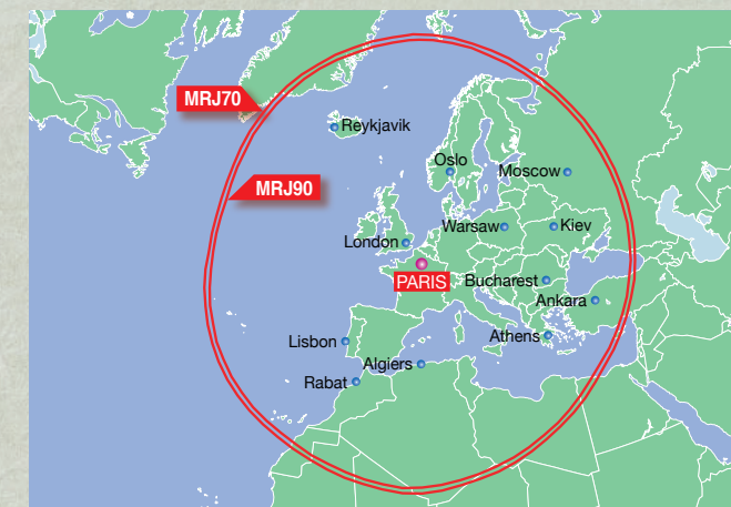
ISA, 85% Annual Wind, LRC @37,000ft, Alternate 200nm Payload : MRJ90 92PAX x 102kg (225lb), MRJ70 78PAX x 102kg (225lb)
