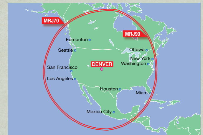
ISA, 85% Annual Wind, LRC @37,000ft, Alternate 200nm Payload : MRJ90 92PAX x 102kg (225lb), MRJ70 78PAX x 102kg (225lb)
