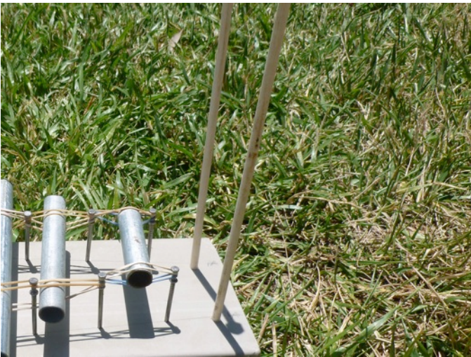
Push the dowels into the holes in the baseboard.
