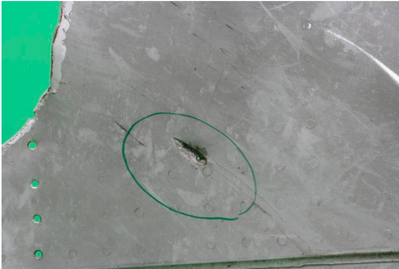
Figure 6: Ricochet damage (Source: DSB)
