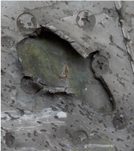
Figure 9: Outer layer penetration
