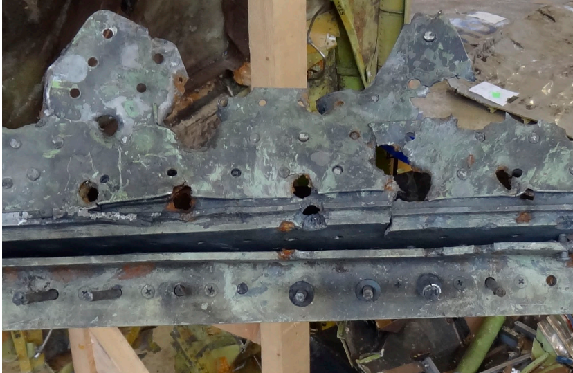
Figure 15: Regularity of hits on upper cockpit window frame
