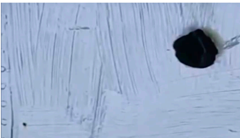
Figure 39: GSh-30 projectile damage detail (Source: YouTube)
