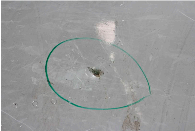
Figure 22: Detail of left-hand side panel ricochet damage
