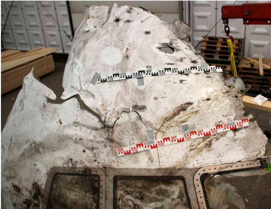
Figure 26: Rulers showing local direction of ricochet damage on cockpit roof
