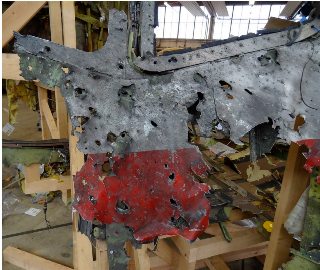
Figure 12: Piece of wreckage used for size of penetration measurement
