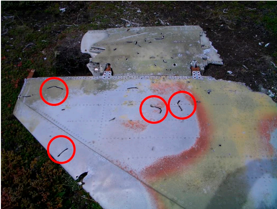
Figure 44: Discrete rod damage (Source: PPRuNe.org)
