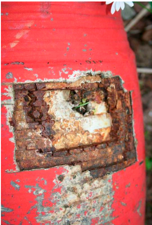
Figure 48: 9N314M warhead fragment layers in an inert warhead. (Source: photo.quip.ru)
