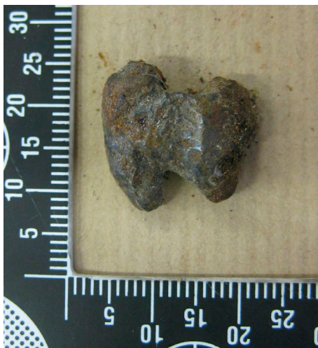
Figure 46: Bowtie fragment found in the wreckage of the cockpit, size in mm (Source: DSB)
