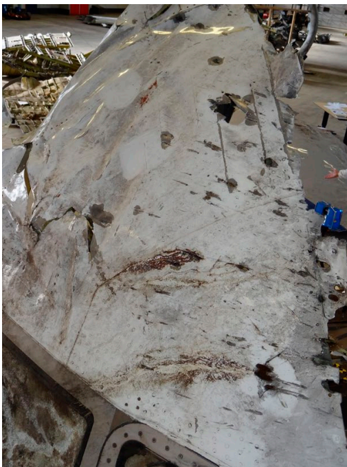
Figure 56: Matching of high-energy object impacts on cockpit roof
