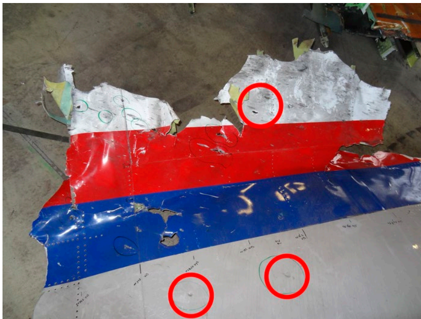
Figure 21: Left-hand side panel with ricochet damage
