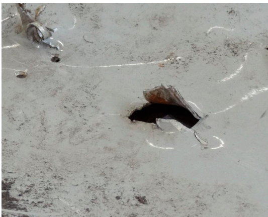
Figure 10: Exit damage on lower right-hand side of the cockpit
