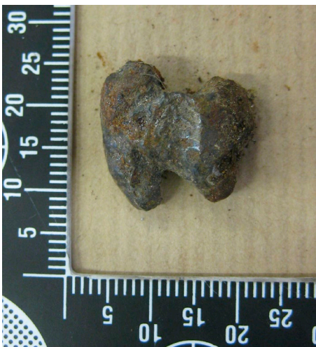
Figure 32: Bowtie fragment found in the wreckage of the cockpit, size in mm (Source: DSB)
