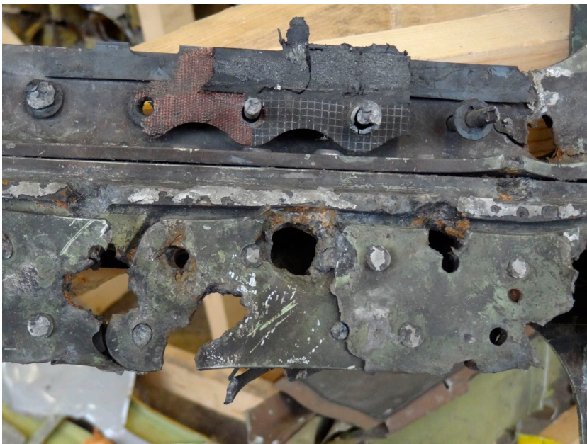
Figure 16: Regularity of hits on lower cockpit window frame
