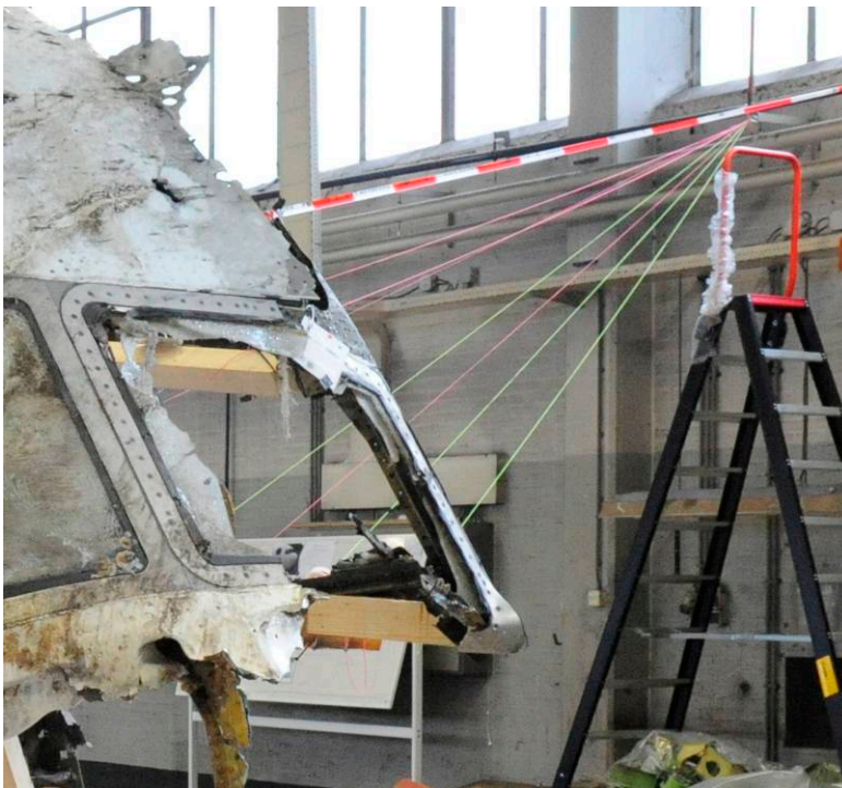
Figure 25: Stringing of high-energy objects impacts to determine general location of origin (Source: DSB)
