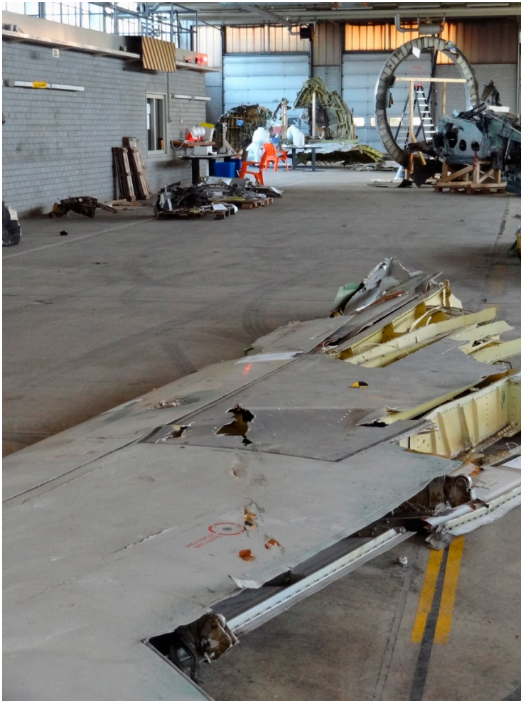
Figure 30: Damage to left wingtip
