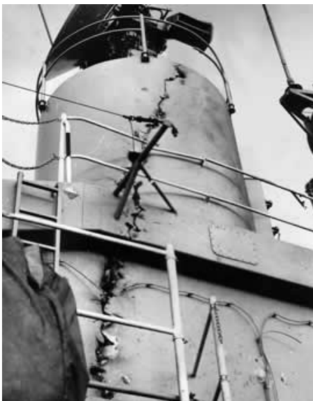
Figure 43: AIM-7 Sparrow continuous rod warhead damage (Source: navalofficer.com.au)
