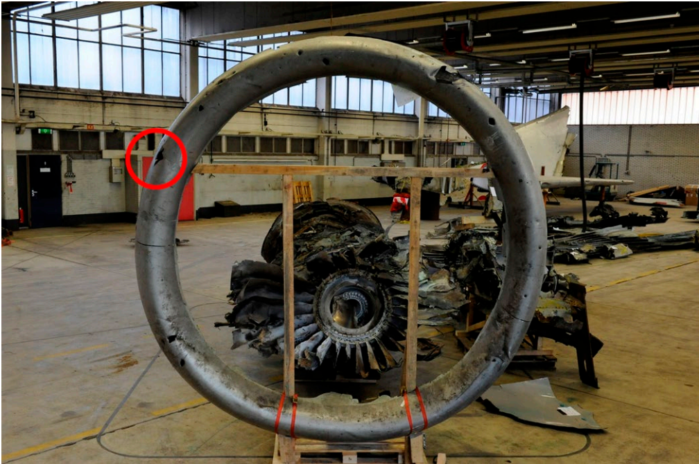
Figure 28: Impact damage on front side engine cowling ring
