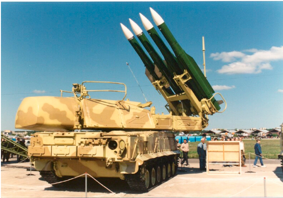
Figure 45: BUK-M1-2 Surface-to-Air Missile System Transporter Erector Launcher and Radar (TELAR) 9A310M1-2 with two 9M317 missiles (left) and two 9M38M1 missiles (right)
