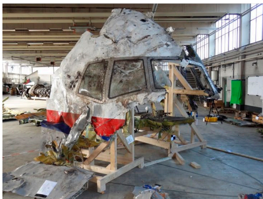
Figure 59: Matching of high-energy object impacts, front view
