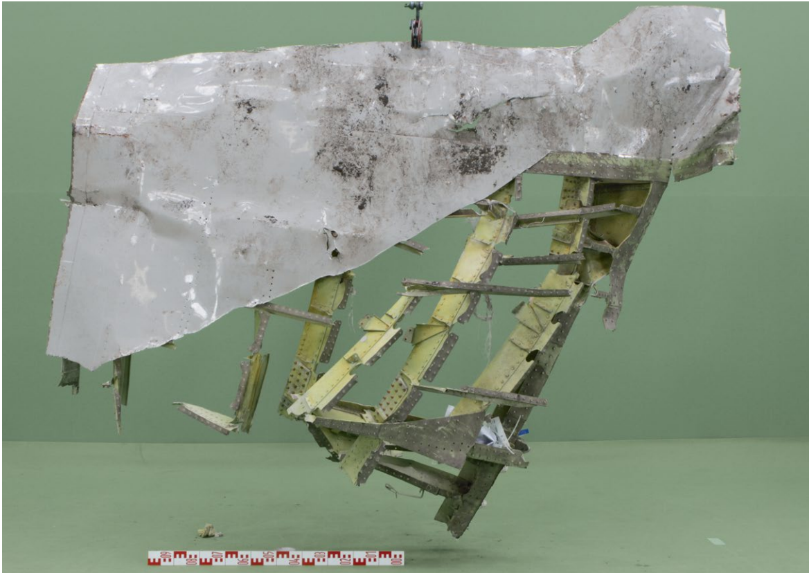
Figure 25: Typical case of skin/sub-structure separation. The skin has been pulled away from stringers and frames. (Source: Dutch Safety Board)
