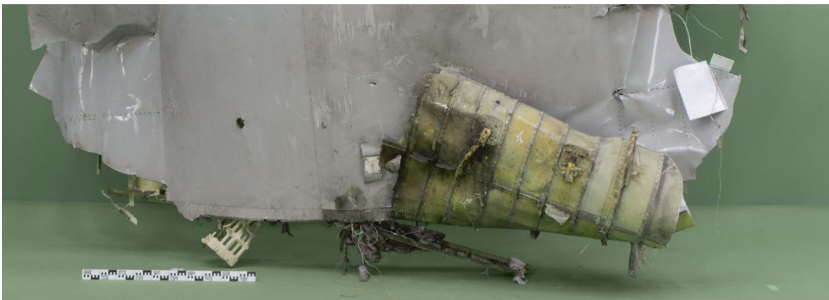
Figure 24: Example of bending/peeling at a fracture line associated with the final separation between two pieces of wreckage. (Source: Dutch Safety Board)
