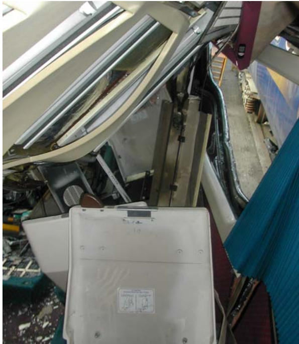
Figure 17 - Structural Intrusion at Ufton Nervet
