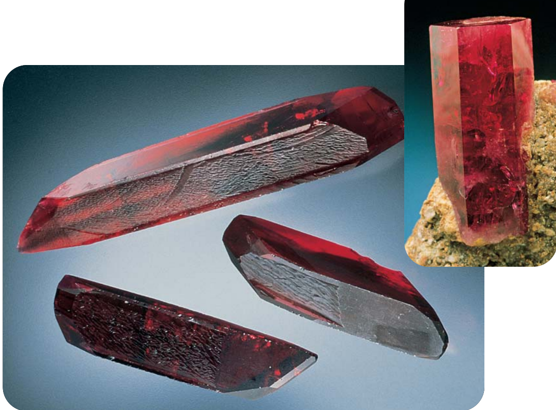
Figure 3. The morphology of these synthetic red beryl crystals (125.7–323.9 ct) differs significantly from the hexagonal crystal form of natural red beryl (see inset, 2.1 cm tall; photo by Jeff Scovil). Photo © GIA and Tino Hammid.
