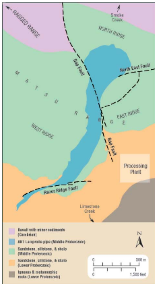
Figure 4. The tadpole-like shape of the Argyle AK1 lamproite pipe, which is broadest to the north and narrowest to the south, is evident in this simplified geologic map. The pipe is located within resistant rocks of the Matsu Range that here form the East and West Ridges.
