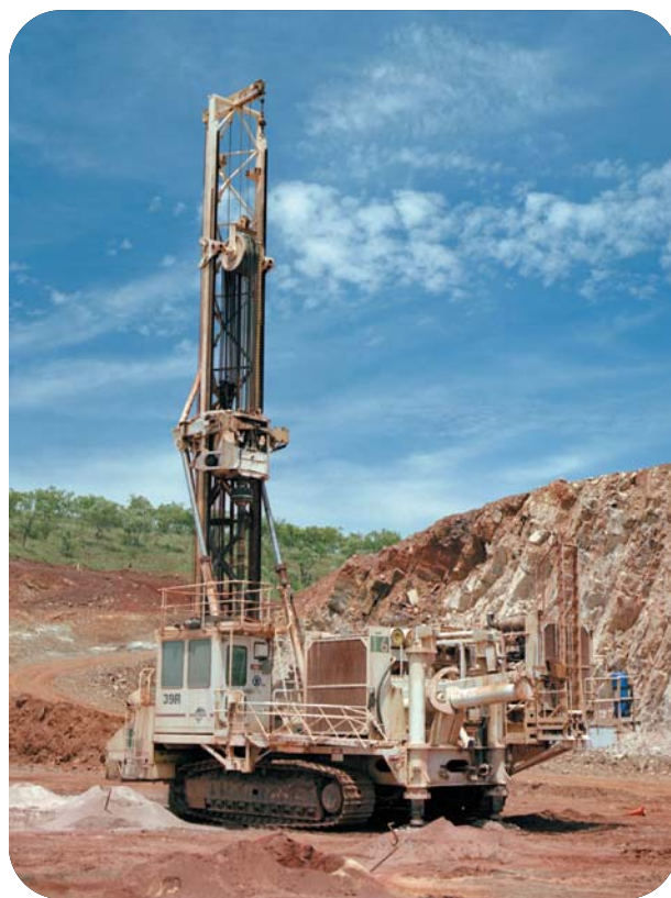
Figure 8. Mobile drill rigs at Argyle make holes for the explosives needed to mine the ore.
