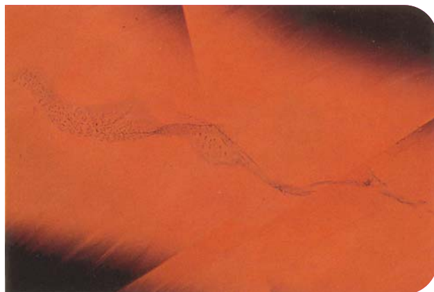
Figure 9. Some synthetic red beryl samples contained small, partially healed fractures composed of numerous tiny liquid or liquid-and-gas inclusions along lines or forming small “fingerprint” patterns. Although often planar, some partially healed fractures displayed curved shapes. Photomicrographs by James Shigley; magnified 8 \times (left) and 14 \times (right).
