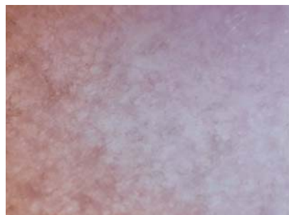
Figure 17. At 50× magnification, the dye concentrations in the bracelet shown in figure 16 can be seen to overlap where the colors appear to meet.
