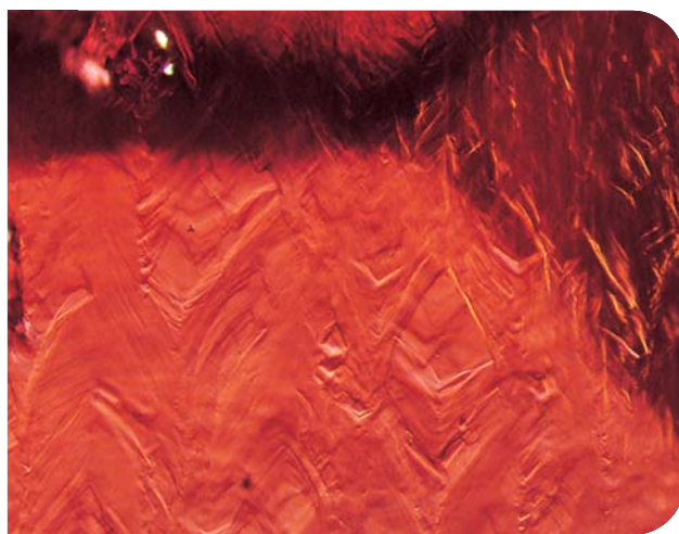
Figure 6. The most distinctive visual feature of the hydrothermal synthetic red beryls examined was chevron-like internal growth zoning. From observations in the original crystals, we know that this zoning is oriented along the direction of crystal growth at a high, oblique angle to the plane of the seed plate. Photomicrographs by James Shigley; left—magnified 3 \times , right—magnified 9 \times .
