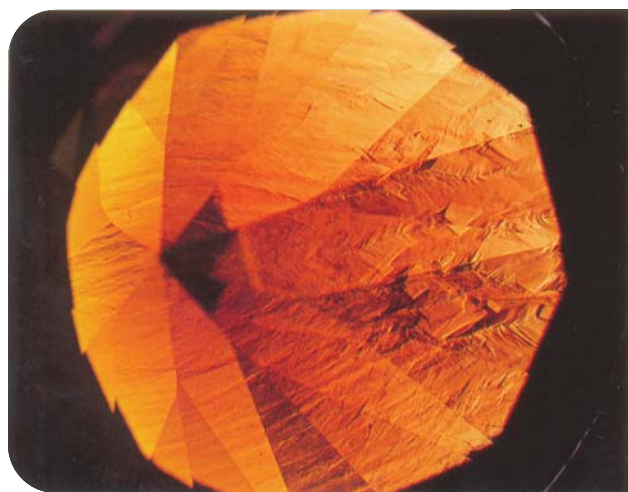
Figure 6. The most distinctive visual feature of the hydrothermal synthetic red beryls examined was chevron-like internal growth zoning. From observations in the original crystals, we know that this zoning is oriented along the direction of crystal growth at a high, oblique angle to the plane of the seed plate. Photomicrographs by James Shigley; left—magnified 3 \times , right—magnified 9 \times .
