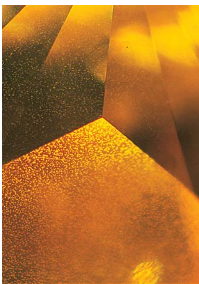
Figure 12. Note the cloud of small highly reflective flux inclusions in this 0.75 ct orange-yellow synthetic diamond. Magnified 30×.
