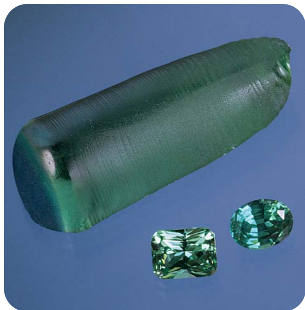
Figure 23. These green flame-fusion synthetic sapphires were reportedly grown in Europe. The faceted examples weigh 2.17 and 1.80 ct, and the split boule measures 40 × 16 mm. Note the dark blue area on the left end of the boule. Courtesy of Lannyte; photo by Maha Tannous.
