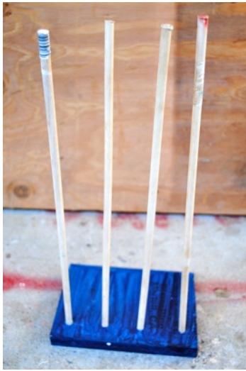
Hammer dowels into the holes in one wood piece.
