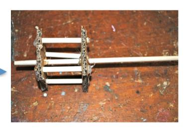
Insert the remainder of the dowel through center of cube. Glue all dowel-cardboard joints tightly.
