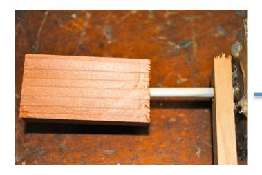
Drill a 19/64" hole in the remaining 1x2 and hammer dowel in to attach the handle.
