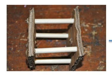
Cut four dowels 2.5" long and stick one in each corner hole to connect the squares. They can't stick out much on the ends.
