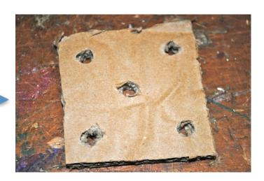
Drill holes in 4 corners and center of each square.
