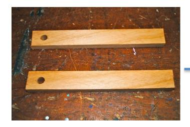
Drill a 3/8" hole at one end of each 7" piece of wood.
