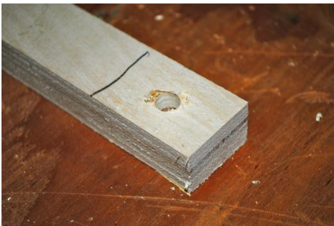
Drill a hole at each end of the rectangular block of wood.
