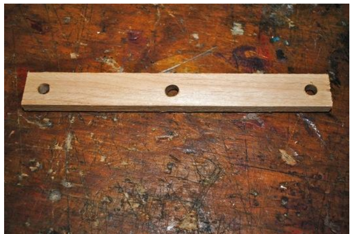
Drill a hole that is wider than the dowel in the center of the block.
