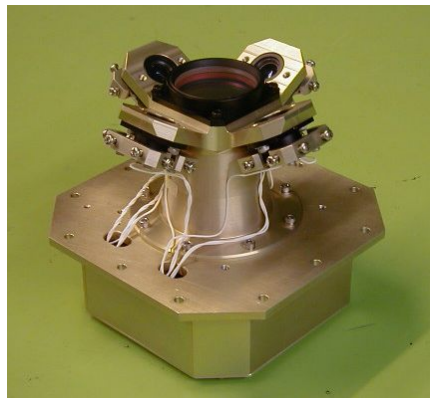
Short-range laser sensor (120m to 3m)
