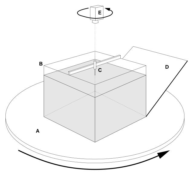
Figure 3. Illustration of experimental apparatus (not to scale). A: Rotating table.B: Lucite tank containing fresh water. C: Reservoir/nozzle apparatus containing dyed saline water. D: Angled mirror to present elevation view to camera. E: Co-rotating video camera.
