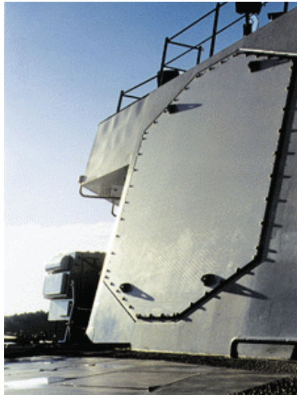
An SPY-1 radar antenna
