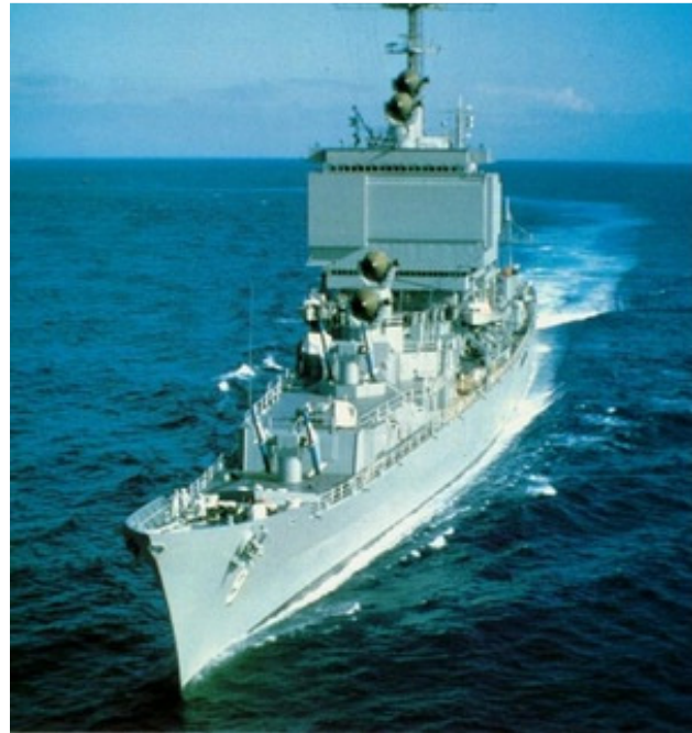
The characteristic antennas of the SPG-32/33 radars are evident in this 1970's shot of the cruiser Long Beach. Note the four separate missile illuminators
