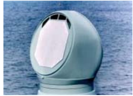
A refined artist's impression of the SAMPSON radar. The antenna shape has been compacted in order to fit in a spherical radome
