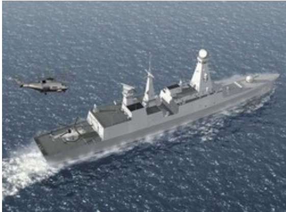
A CGI illustration of a Type 45 destroyer. The SAMPSON figures prominently on the front mast. Notice also the supplementary air-surveillance radar on the third mast
