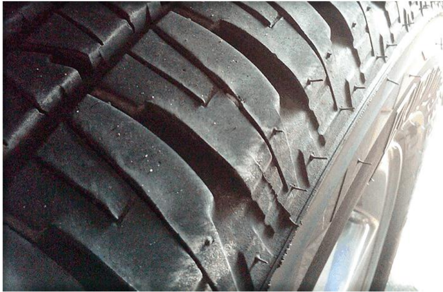
Figure 3: Tire Shoulder View Example 2 - "NORMAL" Tire "Feathering" Wear
