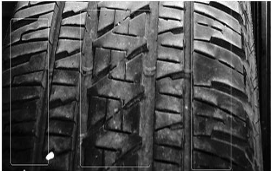
Figure 2: Tire Shoulder View Example 1 - "NORMAL" Tire "Feathering" Wear on the Shoulder
