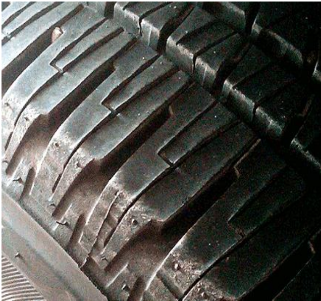
Figure 4: Detail Side View of Tire Shoulder Area - "NORMAL" Tire "Feathering" Wear
