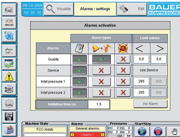
Various alarm settings can be selected by the user.
