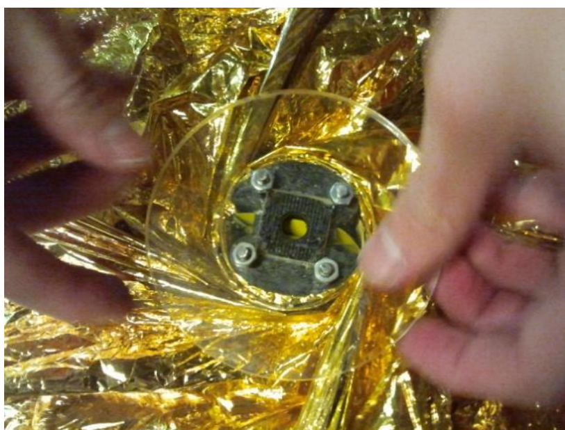
Figure 4-4 Mounting of the flat spring inside the reel.
