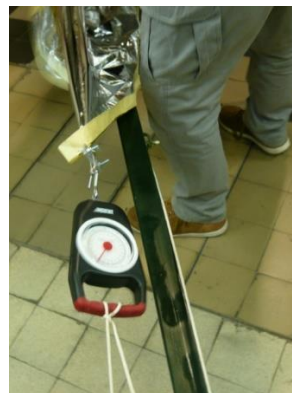
Figure 4-21 Jaxon WA120 scale and its mounting to stand's arm with the line
