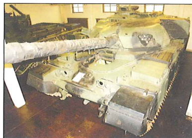
Above: this Chieftain Mk. 10 arrived in Sweden in 1993 in exchange for a Stridsvagn 103. The British registration number was 03 EB 67. Originally, the tank was a Mk. 2, upgraded to Mk. 6/2 and then later to a Mk. 10 with Stillbrew armour.
