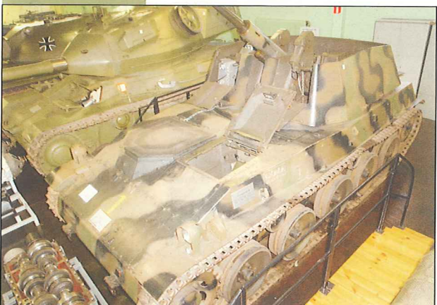
Top left: the Luftvärns-robotbandvagn 701 is an Infanteri-kanonvagn 102 or 103 converted to a self-propelled anti-aircraft vehicle armed with Robot 70 missiles. 48 such conversions were made.
