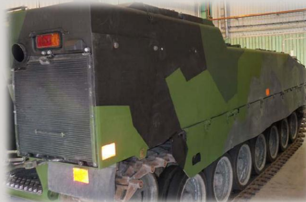
Extended roof 170 mm at the rear
