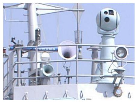
INS Car Nicobar - Close up of the EO turret. Furuno navigation radar also visible.
