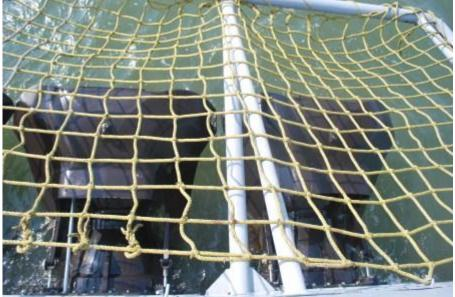
Two of the three HamiltonJet HM811 Water Jets of the INS Cankarso. The Cankarso is a Water Jet Fast Attack Craft (FAC). The propellers are actually fitted inside pipes through which water is pushed out at high speed. This also makes the Water Jet FAC much quieter. (<u>Stratpost</u>)
