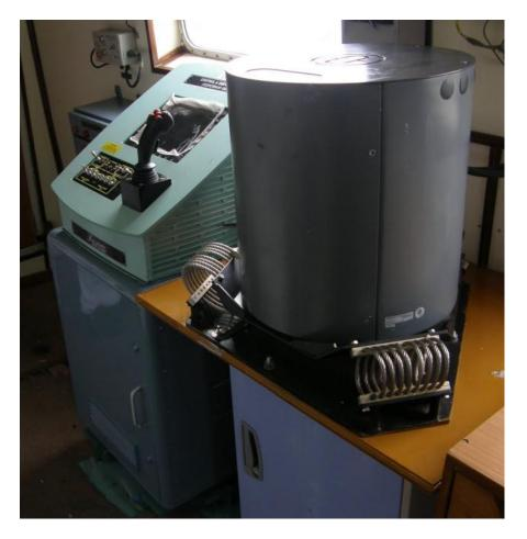
The gun controls for the CRN 91 cannon, and the spring-mounted gyro in the bridge (<u>Broadsword</u>)
