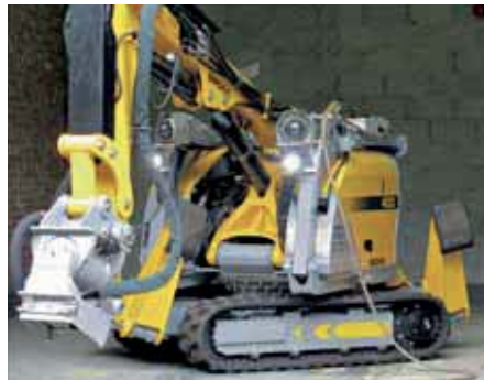
Brokk for retrieving FED
