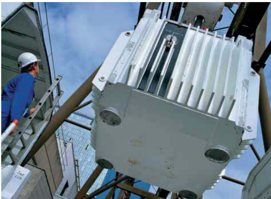
Movement of a Magnox fuel transport flask
