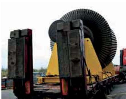
Turbine rotor sent for recycling
