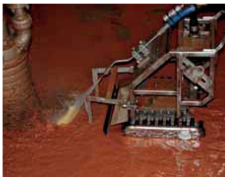
Trawsfynydd's ROV retrieving sludge from resin vault one
