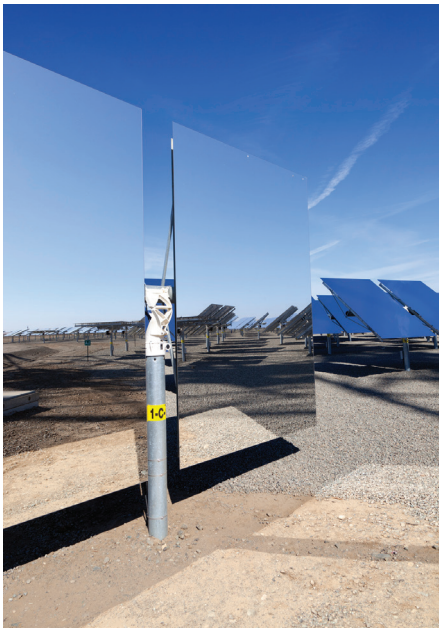
BrightSource's heliostats, consisting of two 12x7 foot, flat-glass mirrors and minimal steel, are individually controlled and optimized to accurately reflect the sun's energy onto the tower receiver.
