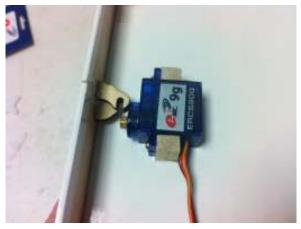
4. Use wood screws to secure the servo.
