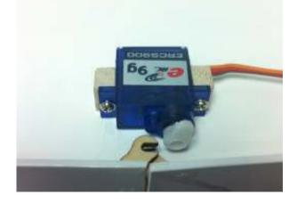
9. Move the gear switch and adjust the gear channel end point so the arm does not bind and looks like the photo.
