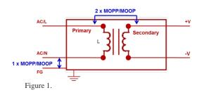
The isolation, creepage and insulation requirement for MOPP and MOOP are different and provided in Table 1.
