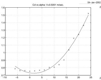
Figure 4: Hull Drag:  $C_D$  versus  $\alpha$ , V=0.5m/sec. a=5.25 rad.<sup>-2</sup>, b=-0.315 rad.<sup>-1</sup>, c=0.732
