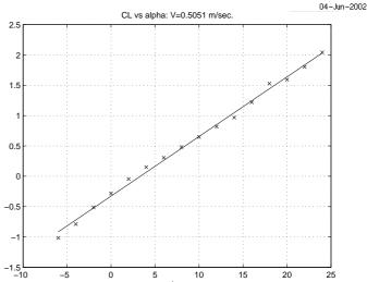
Figure 5: Hull Lift:  $C_L$  versus  $\alpha$ , V=0.5m/sec. Slope:  $C_{L_{\alpha}}$ =4.79 rad.<sup>-1</sup>
