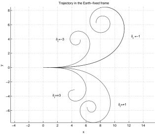
Figure 11: Simulated trajectory at various rudder angles V=1.54 m/sec.,  $K_p$ =-0.543 Nm
