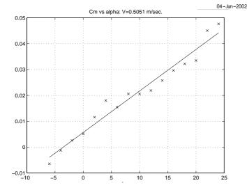
Figure 6: Hull Moment:  $C_m$  versus  $\alpha$ , V=0.5m/sec. Slope:  $C_{m_{\alpha}}$ =0.0974 rad.<sup>-1</sup>
