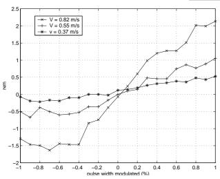
Figure 9: Fin Rolling Moment: Rolling Moment vs aileron angle, V=[0.37, 0.55, 0.82] m/sec. NB:  $|K_{uu\delta_s}| = |K_{uu\delta_r}| = \frac{|slope|}{4V^2}$
