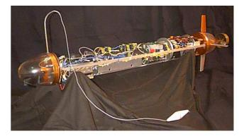
Figure 2: Torpedo shaped AUV: casing removed
