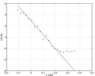
Figure 7: Fin Lift: Lift vs  $\delta_r$ , V=0.81m/sec. NB:  $|slope| = 2 |Y_{uu\delta_r}| V^2$ =-25 N.rad.<sup>-1</sup>
