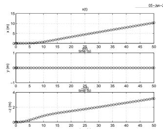
Figure 13: Simulated trajectory as the unpowered submarine surfaces.
