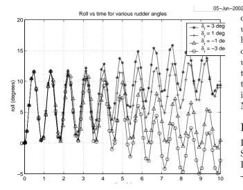
Figure 12: Simulated roll vs time at various rudder angles.
