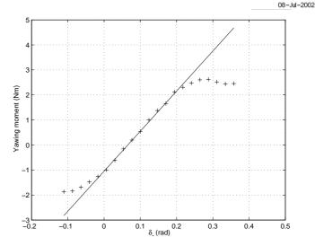
Figure 8: Fin Turning Moment: Moment vs  $\delta_r$ , V=0.81m/sec.  $|slope| = 2 |N_{uu\delta_r}| V^2$ =16 Nm.rad.<sup>-1</sup>
