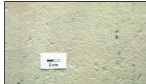
Figure 6b. Close-up of Cockeysville Marble used in the low stone wall surrounding the Battle of North Point Monument (Stop 6).
