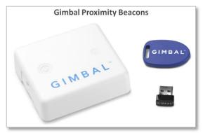
The primary purpose of a beacon is to send a signal via Bluetooth that can be detected by mobile devices in the vicinity of the beacon. When a mobile app programmed to recognize the beacon's signal comes within a specified distance (e.g., from within inches to up to 50-75 meters), the app "wakes up," detects the beacon's presence, and based on intelligence in the app and/or cloud displays a message, ad, offer or other communication on the user's device.
