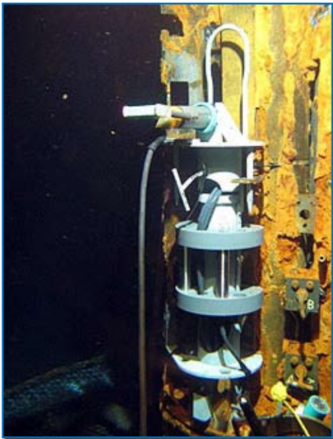
A pressure data logger installed on a CORK at ODP Site 1026B.
