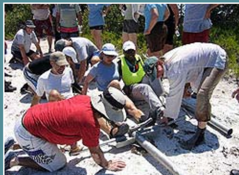
Vibracoring in the southern tidal inlet. Photo Credit: Christian Strohmer (ExxonMobil)
