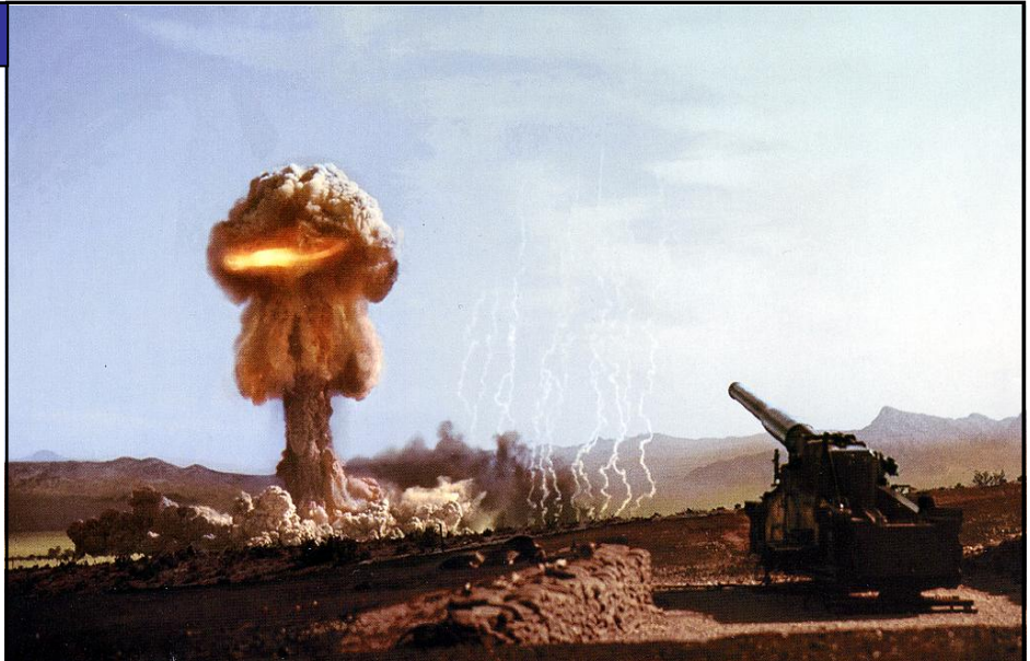
Mk-65 280mm Atomic Cannon fired 15 kiloton nuclear projectile that detonated 8 miles downrange at Frenchman Flats, Nevada
