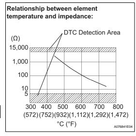
4. High or Low Impedance of Heated Oxygen (HO2) Sensor (DTCs P0136 and P0156 or P0137 and P0157)
