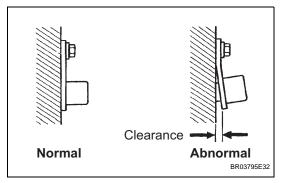
(a) Check the CKP sensor installation.
