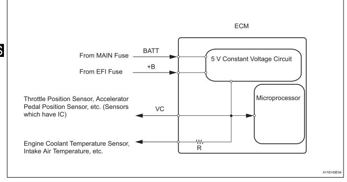
When the VC circuit is short-circuited, the microprocessor in the ECM and sensors that are supplied power through the VC circuit are inactivated because the power is not supplied from the VC circuit. Under this condition, the system does not start up and the MIL does not illuminate even if the system malfunctions.
