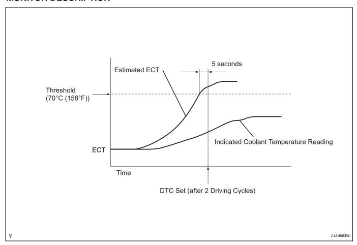
The ECM estimates the ECT based on the starting temperature, engine loads, and engine speeds. The ECM then compares the estimated temperature with the actual ECT. When the estimated ECT reaches 70°C (158°F), the ECM checks the actual ECT. If the actual ECT is less than 70°C (158°F), the ECM interprets this as a malfunction in the thermostat or the engine cooling system and sets the DTC.
